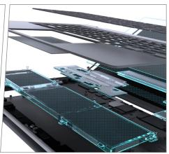
ASUS BR1100 has a modular design that allows key components — such as the keyboard, battery, thermal module and I/O ports — to be replaced in minutes using simple tools.
