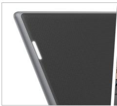
LED indicator status — On: Normal operation; Slow blinking: Less than 20% battery power remaining; Fast blinking: No WiFi or 4G connection.
